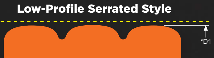
Fig. 5 - Low-Profile Serrated Style (*D1 = Tool Cutting Diameter)
